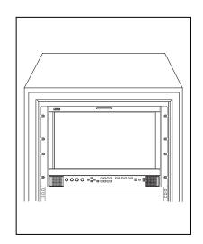
Step1: Fix the supplied rack ears onto left and right side of the DT-G17E monitor, by supplied 4 screws. Step2: Install the monitor onto the standard 19-inch rack. Occupy 7U height.
