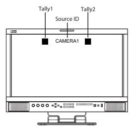
Source ID letters by manually input, Tally1/Tally2 input via GPI pin assignment.
